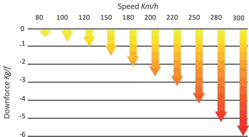
The Downforce that the spoilers generates raises potentially as the speed increases, at 300 km/h we get 5.9 Kg/f.
